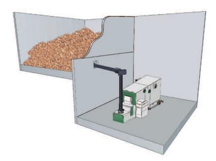
Storage room and heating room are on different levels. Horizontal discharge with spring agitator and falling chute.
