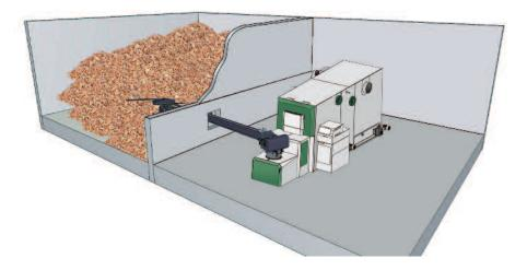
Storage room and heating room are on same level. Transverse discharge with spring agitator.
