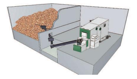
Room discharge via horizontal spring agitator and connected feed screw for optimum use of the storeroom. This arrangement enables greater flexibility of boiler location.
