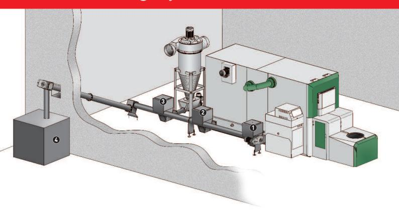
Ash discharge using a screw:
