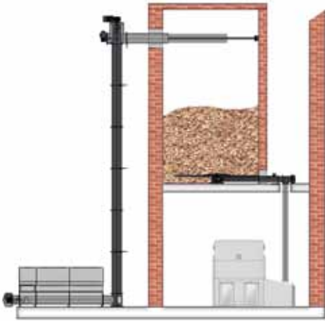
The storage room is located above the boiler room
